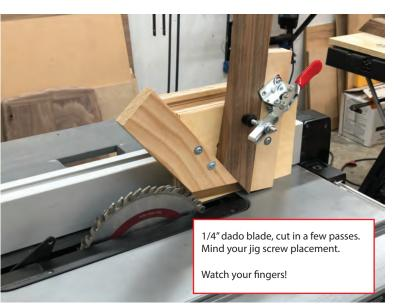
Here's my on-the-cheap jig for cutting the bridle miter. Both this jig and the one for the vertical leg pieces ride on a saddle that fits over the table saw fence.
