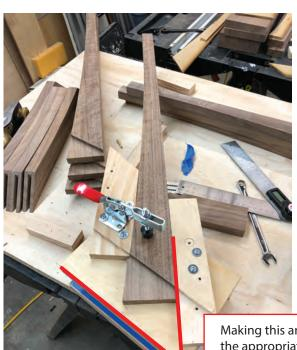
Cut all legs on one side first, then adjust fence and cut away inner 1/4" using saddle as a sacrificial fence.
